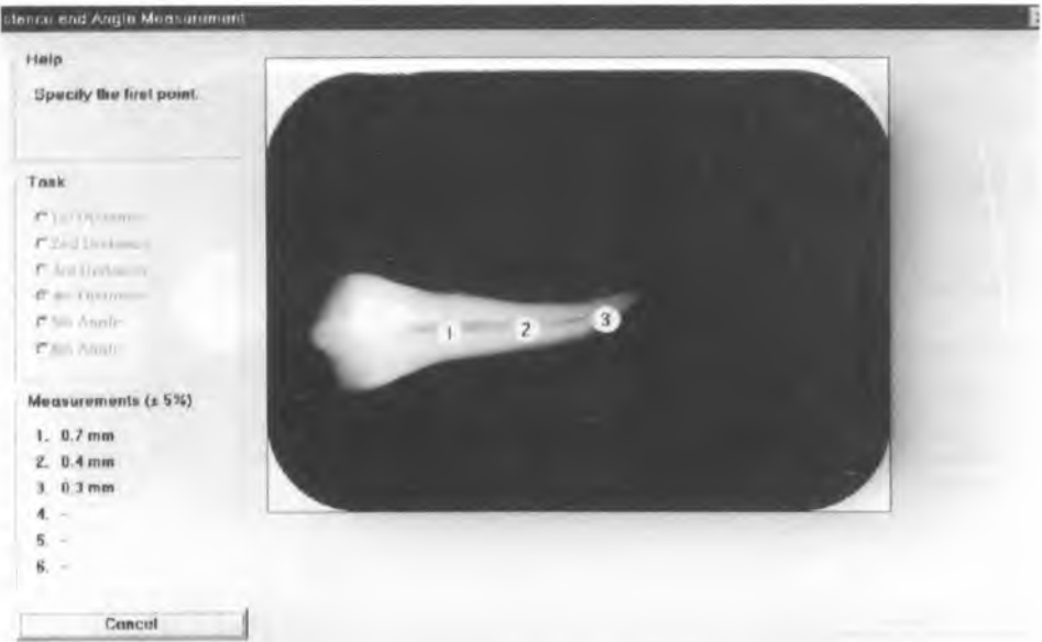
Fig. 3. Another second maxillary premolar in the mesiodistal projection with root canal width measured at 5, 10 and 15 mm coronal from the radiological apex
